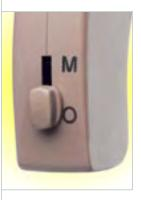
Your BTE has a two position switch to turn the instrument "on" and "off." To turn BTEs "on," move the switch to the "M" (microphone) position. To turn the instrument "off," move the switch to the "O" position.
